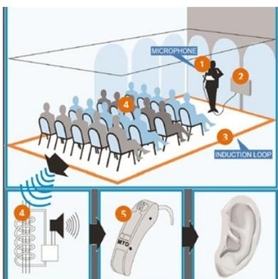
The basic technology, called an induction loop, has been around for decades as a means of relaying signals from telephones to Telecoil receivers in hearing aids. European countries have required use of Telecoil systems in public areas for many years where they are connected to microphones in halls, stores, taxicabs, and many other venues. In the USA, Telecoil systems have recently been installed at ticket windows of many sports stadiums, Broadway theaters, and even in the New York Subway system!
